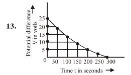
The figure shows an experimental plot for discharging of a capacitor in an R-C circuit. The time constant  $\tau$  of this circuit lies between:
