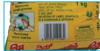
**Cylindrical products:** Close to the natural base of the product. The barcode should be in ladder orientation with human readable number on the left.
